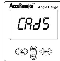
7) Turn the box another 90 degrees clockwise; press the ZERO button—the screen will read CAD5. After 3 seconds the display will read 0.00—this completes the calibration.
